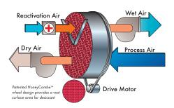
The other air stream dries the rotor so it can absorb moisture again and this accumulated moisture is then exhausted away externally. We deliver cost effective solutions at the highest quality level, that are manufactured under strict control regulations in our ISO 9001: 2008 and 14001 certified facilities. And our systems can be designed according to your requirements.
